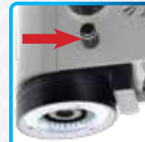
Independent ring light adjustment knob
