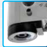
LED Ring light with quadrant control
